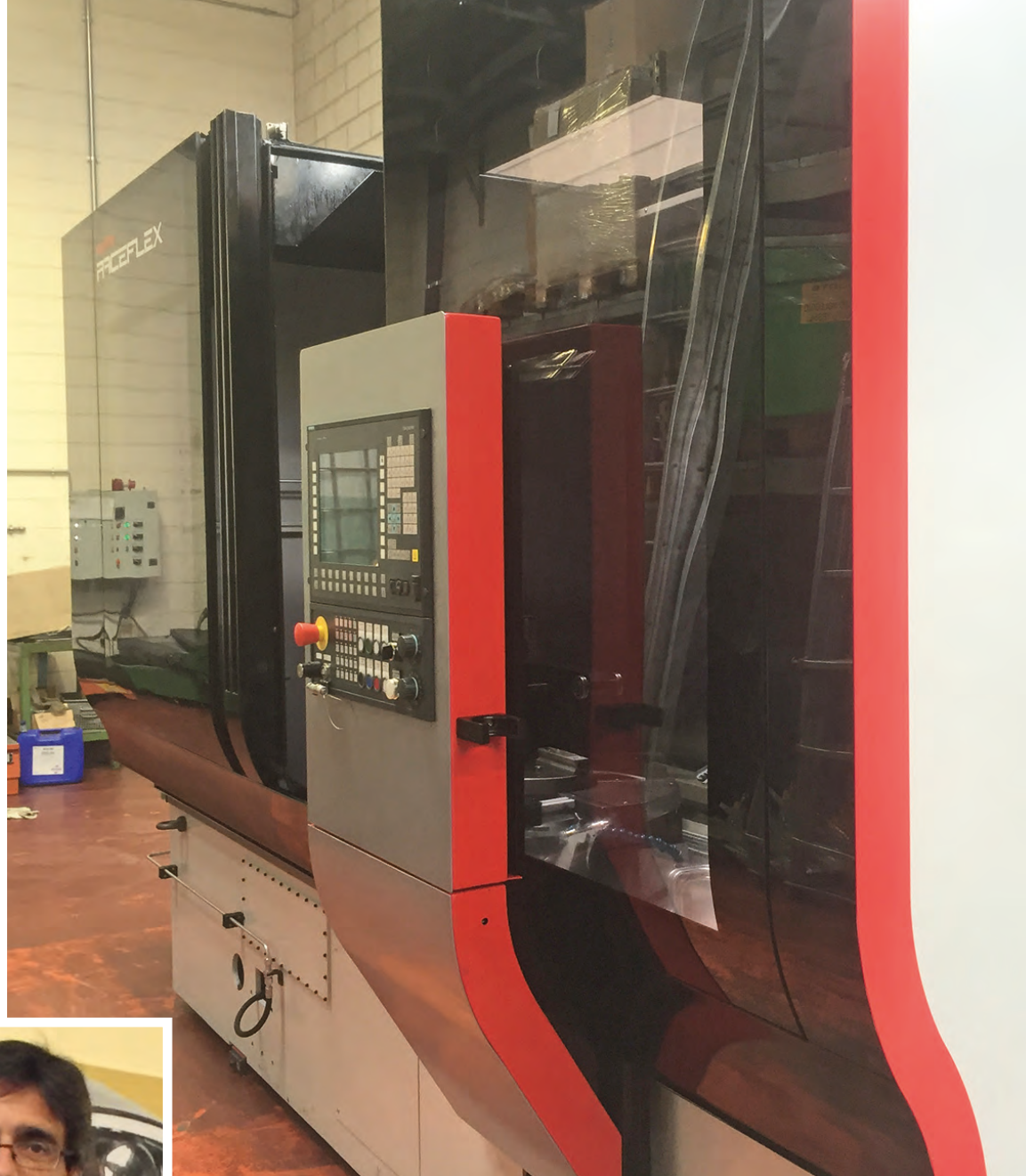
Lapping machine for rolling raceways.
